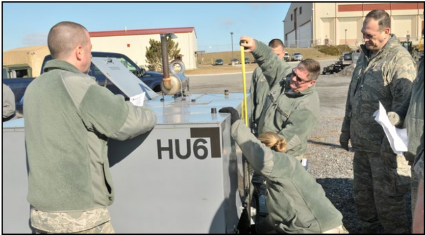
(Above) Senior Master Sgt. Michael Decker shows Airmen how to measure the height of aerospace ground equipment (AGE) that will deploy to Greenland. (Left) Tech. Sgt. Kyle Partlow and Staff Sgt. Jessica Collins measure the wheelbase of AGE equipment. The Airmen were getting training on preparing cargo for deployment which would actually be deploying to Greenland for the start of the season.
