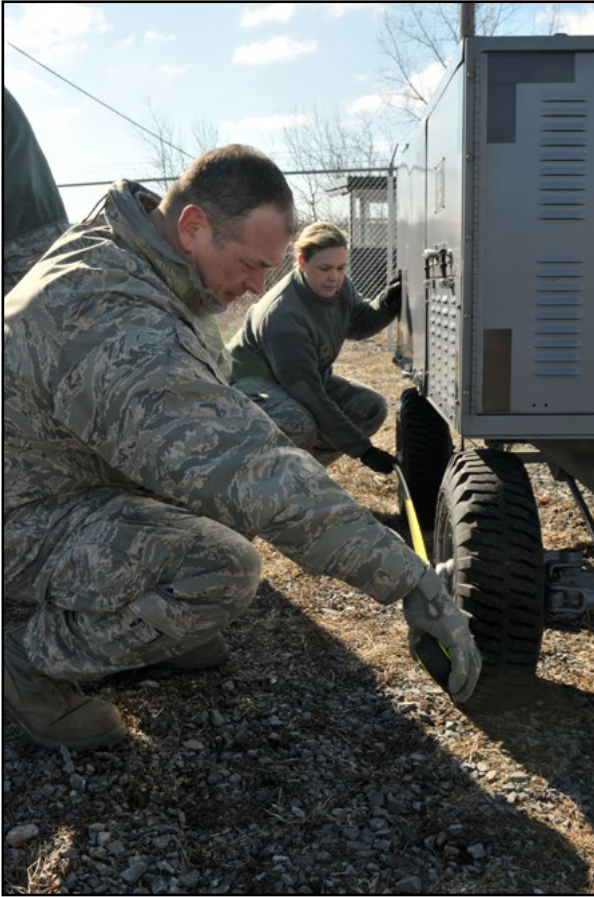
(Above) Senior Master Sgt. Michael Decker shows Airmen how to measure the height of aerospace ground equipment (AGE) that will deploy to Greenland. (Left) Tech. Sgt. Kyle Partlow and Staff Sgt. Jessica Collins measure the wheelbase of AGE equipment. The Airmen were getting training on preparing cargo for deployment which would actually be deploying to Greenland for the start of the season.
